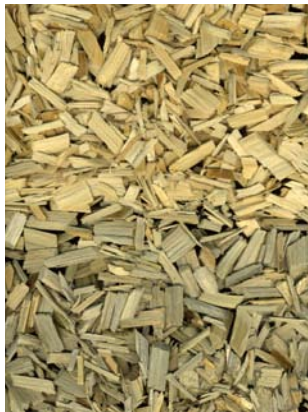
Normal chips (top) and beetle-killed chips (bottom) are fed into the pulp and paper plant.
