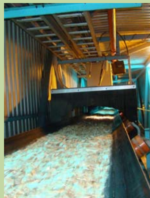
The on-line system uses algorithms to quantify bluestain and brightness
